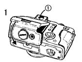
If you record outdoors and the sunlight is strong, it is difficult to see the LCD monitor. In this case, by attaching the supplied monitor hood, you can see well.
